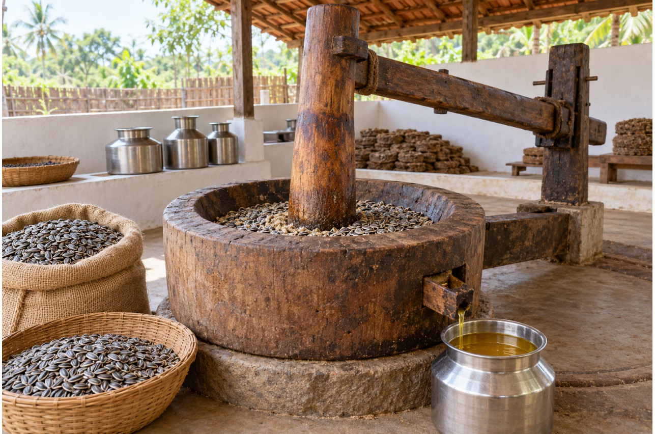
The rotating pestle crushes seed in the mortar; press designs and methods vary.
