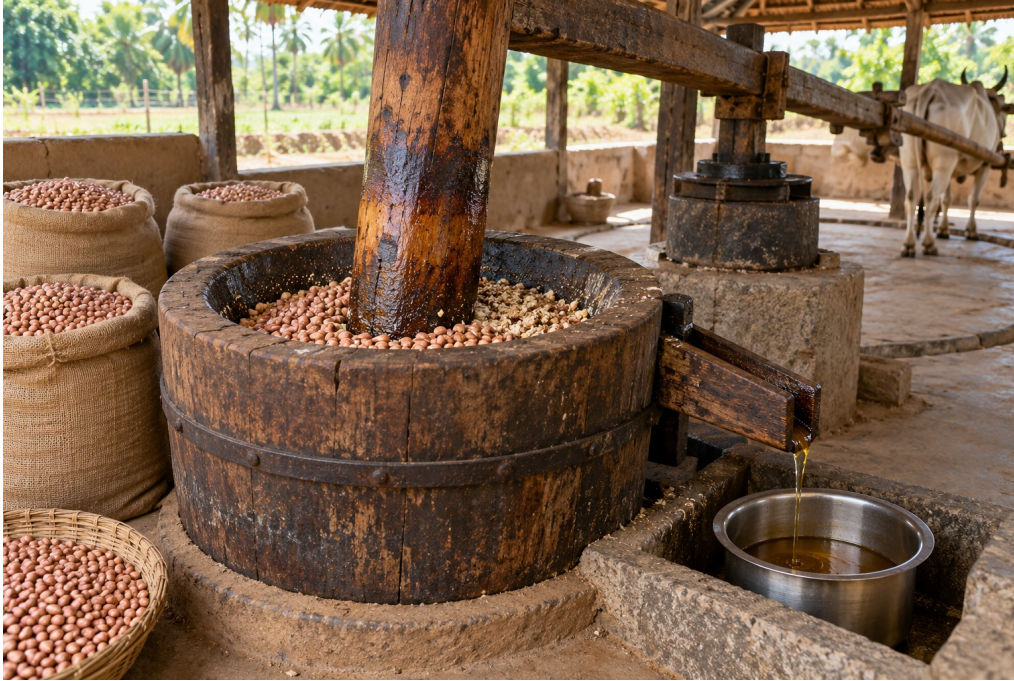
The rotating pestle crushes groundnut kernels; actual press designs and methods vary.
